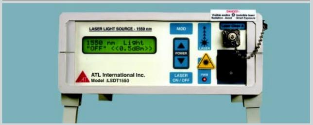
Laser Light Source 1550nm designed and developed by ATL International Inc. is a Stabilized Laser Light Source instrument for field or laboratory testing of fiber optic systems. It features excellent accuracy and high performance source for SMF testing. The RS 232c port is provided for external control using a PC. The instrument is dust proof & drop protected.
